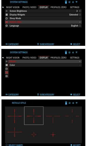
You can manage reticle style in the System Settings (Display section).
