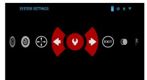
To enter the System Settings, open the Shortcut Carousel by pressing the OK button 💓. Select the wrench icon with RIGHT or LEFT buttons 🖾.
