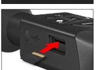
The device is equipped with a microSD Card and USB (type C) ports. You can find them under the rubber caps on the right side of the device (we marked the caps with appropriate icons).
