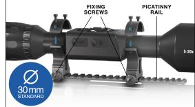
tion and mount the bottom portions of your rings to your rail for optimal eye relief. Place the scope on the bottom half of the rings you just mounted, verifying you have sufficient eye relief for your platform. Place the top portion of your ring over the mounted bottom portion, make sure the holes align and the screws turn easily. Apply equal torque to all screws with the provided Allen wrench. Make sure your rings are tight on your rifles rail and will not come loose due to recoil.
