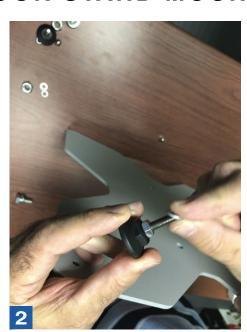
Install the crush washers and washer after nut. As shown in the image.
